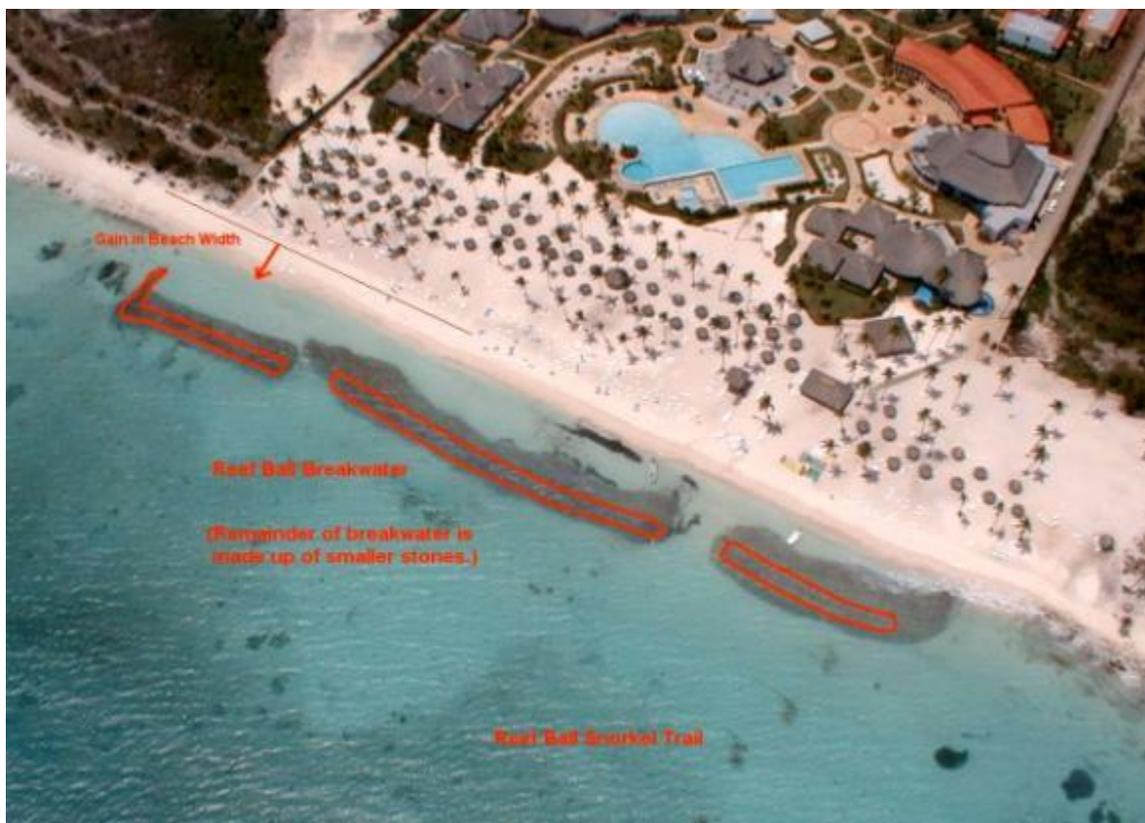
**Figure 8. Deliniation between the original Reef Ball breakwater and smaller rocks.**
